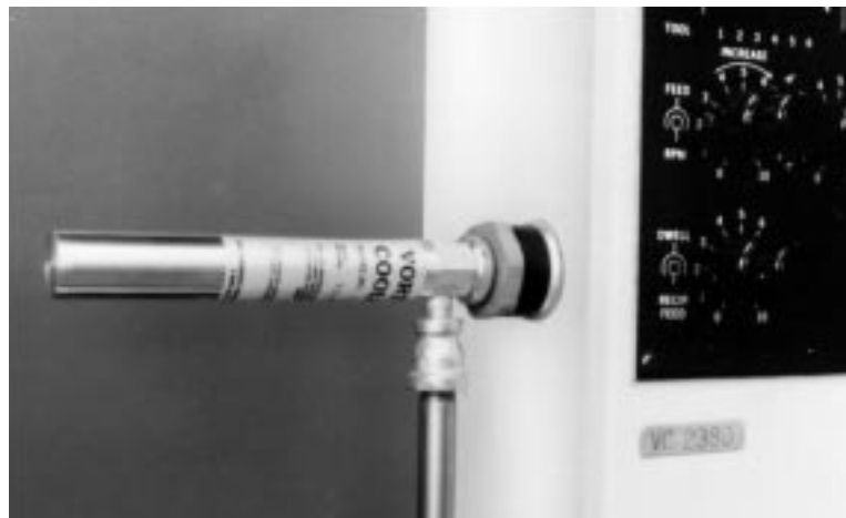
Figure 20-12. Vortex cooler used in cooling systems.
