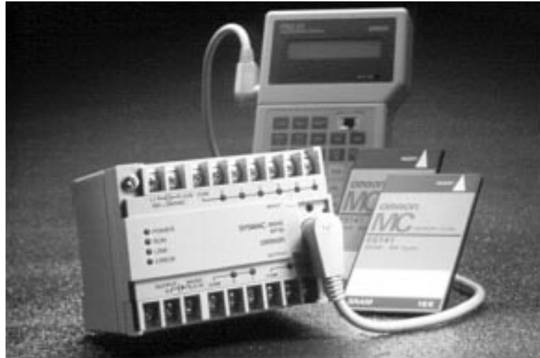
Figure 4-23. A typical miniprogrammer and a small PLC.
