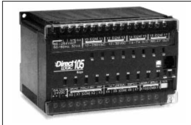
Figure 21-2. PLC Direct's micro PLC DL105.
