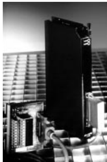
Figure 8-10. Allen-Bradley's Weigh Scale Module (1771-WS).
