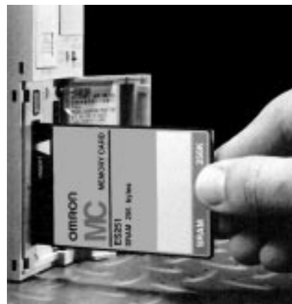
Figure 4-24. A removable memory card for a miniprogrammer.
